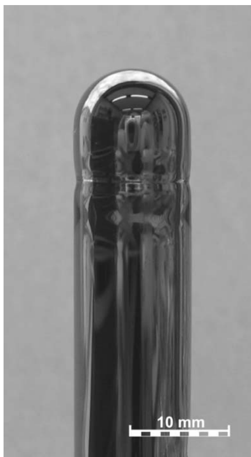
Fig. 7 Picture of the new glass electrode with internal metallic coating
